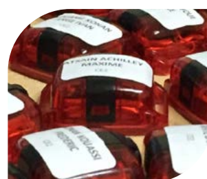
▲ Accelerometers (red devices)
